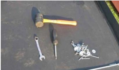
Tools needed – Phillips screwdriver – spanner – also useful to have a rubber or wooden mallet.
